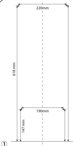
Select a suitable wall on which to mount the unit. Using the unit as a template, mark the position of the 4 holes checking the dimensions (as seen above) afterwards with a tape measure. Drill the wall using an 8mm masonry bit and plug with the wall plugs provided.
